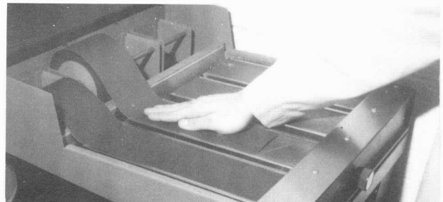
c. Slide the paper across the platen, using the heel of the hand.
