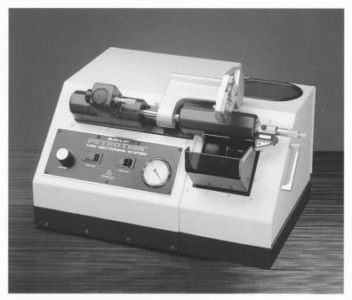
Dimensions and shipping weight for PETROTHIN® Thin-Section System: Overall dimensions: 23"W x 19"D x 12"H (59 x 48 x 30.5 cm) Approx shipping weight: 120 lbs (55 kg)
