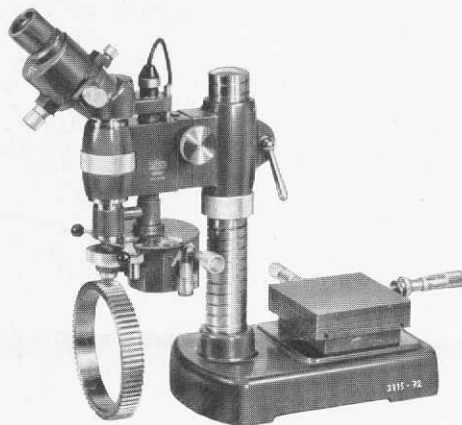
Hardness tester swung around for testing larger work pieces.
