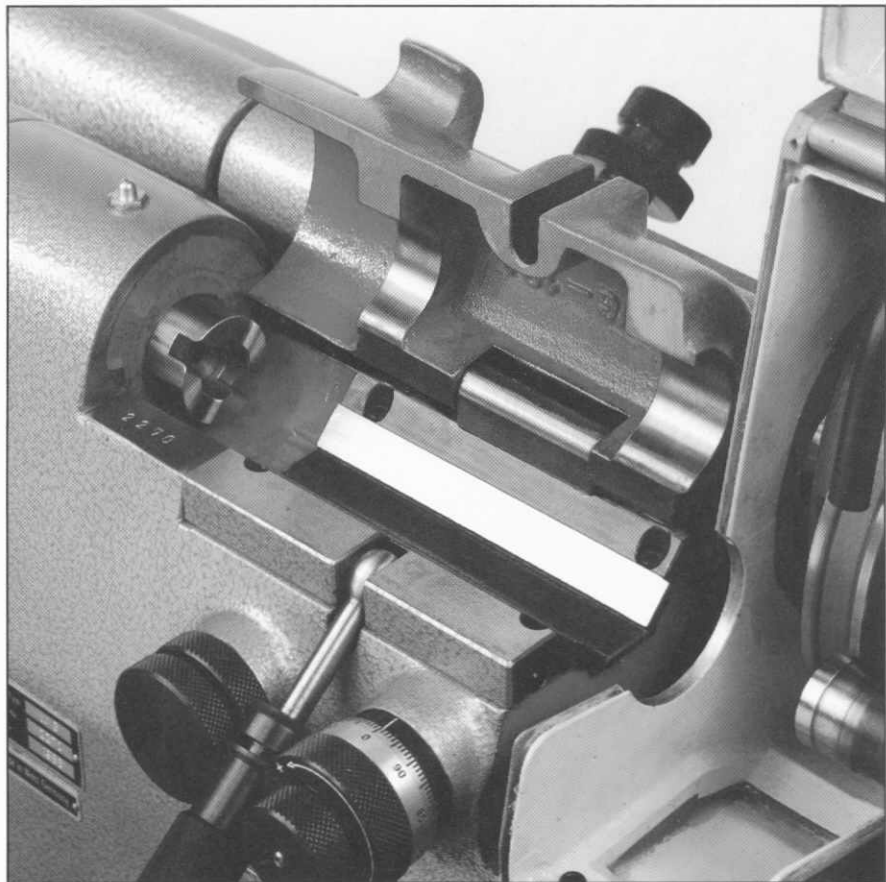
V-blocks for the centering spindle as an option, recommendable for alternating between the cementing and bell clamping method
