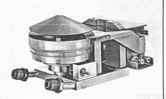
The crucible may be rotated either manually or by motor. As with other Airco sources, the TIH-270 can be precisely controlled and offers exceptional high rate and high purity deposition. Its extremely long filament life, electro-magnetic deflection, standard lateral deflection coil and accurate beam positioning assure reliable performance.
