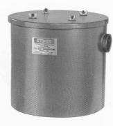
Traps sub-micron oil particles to remove oil smog and solids from pump exhaust. Reduces air contamination. Double cleaning action. Filters particles as small as .03 micron; replaceable element is simple to maintain. All units are closed circuit type. Piping kit for attaching to Stokes pumps included.
