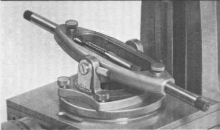
Checking a tap with Model TM-IS Inclinable Stage and Workholder.
