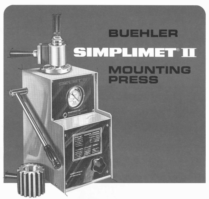
The SIMPLIMET® II Mounting Press utilizes a proven hydraulic system that provides positive compression action for specimen mounting. It produces a full compliment of sample sizes, 1" (2.5cm), 11/4" (3.2cm) and 11/2" (3.8cm), to satisfy virtually any
